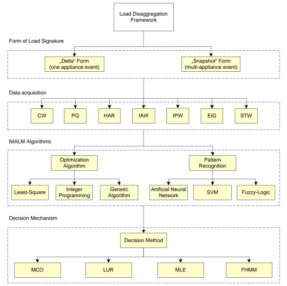
Figure 1: Overview of a load disaggregation framework
