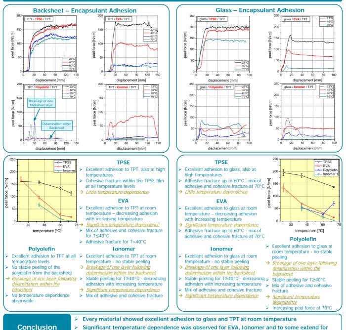
Polyolefin – strong decrease in adhesion to TPT backsheet and glass at temperatures > 40°C
