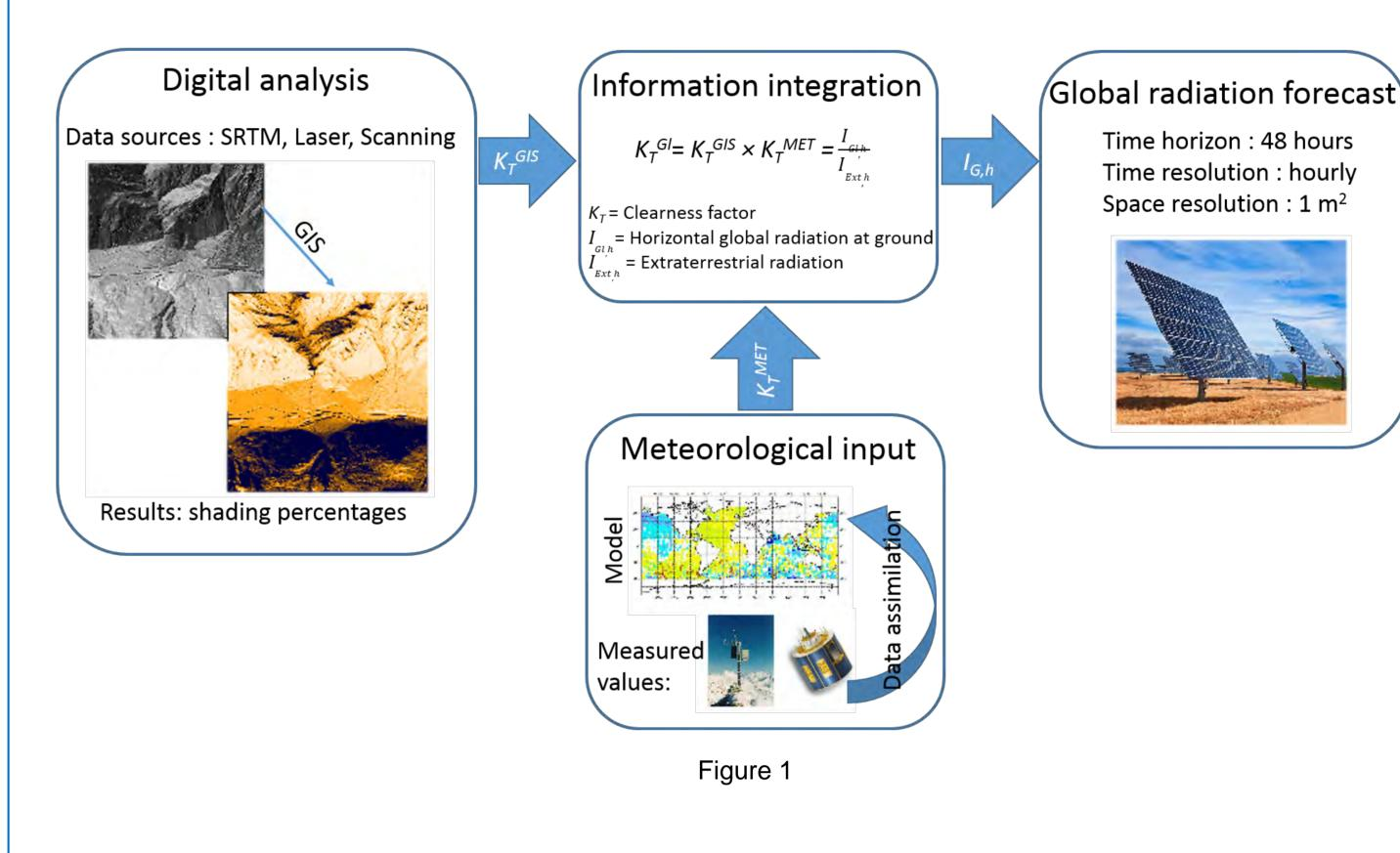
Historical data are collected from different PV installations including power production, ground solar radiation and ambient temperature. Having the solar radiation forecast (figure 1) the historical data are used to extrapolate the power production for other PV installations when no other data is provided.
